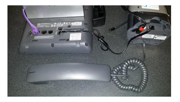
Your phone may have a jack on the back that has a headset symbol (marked in red below). More than likely your existing headset will not work when plugged into this port, plug the headset into the handset port (marked in green below) and then plug the phone's handset into your headset's reciever (pictured above).
