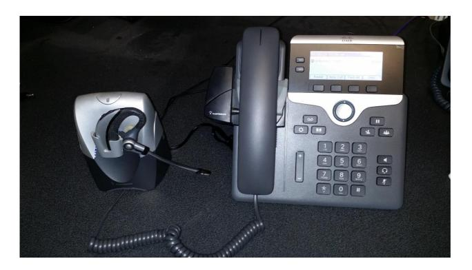
In the testing the OIT has done with the new Cisco VOIP phones we have found the best way to connect a standard external headset to a Cisco VOIP phone is to use the pass-thru method – meaning the headset is plugged in between the phone itself and the handset of the phone as pictured below. Please note: it still is necessary to take the handset off the hook in order for the headset to work, unless you have a hands free headset that will lift the handset off the hook (pictured above)
